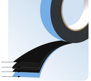
adhesive coating, black, acrylate carrier, PE foam, black adhesive coating, black, acrylate Liner, siliconised PP film, blue
